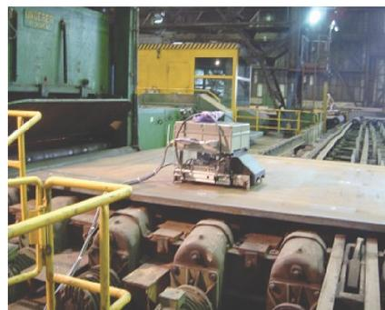
**Heavy steel plate inspection (hardness, mechanical strength) by means of an inspection trolley on the roller table position**
