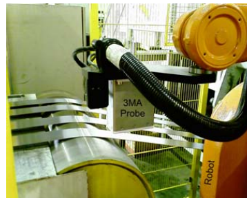
Figure 15 3MA probe with robot at a strip line
