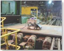
Heavy steel plate inspection (hardness, mechanical strength) by means of an inspection trolley on the roller table position
